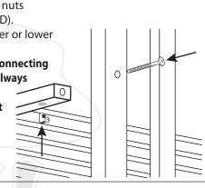
Attach the screws (2) to the lower brackets (4) in the lower part of the legsof both front walls and slide through into the pull-in side (E). Drilled holes metal rods (8), in the middle with threaded middle holders (5)
