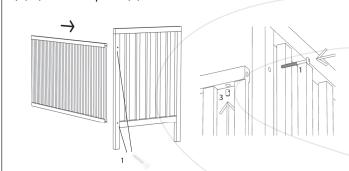
Screws (1) and roller nuts (3) attach the grate (D). You can choose upper or lower position.
